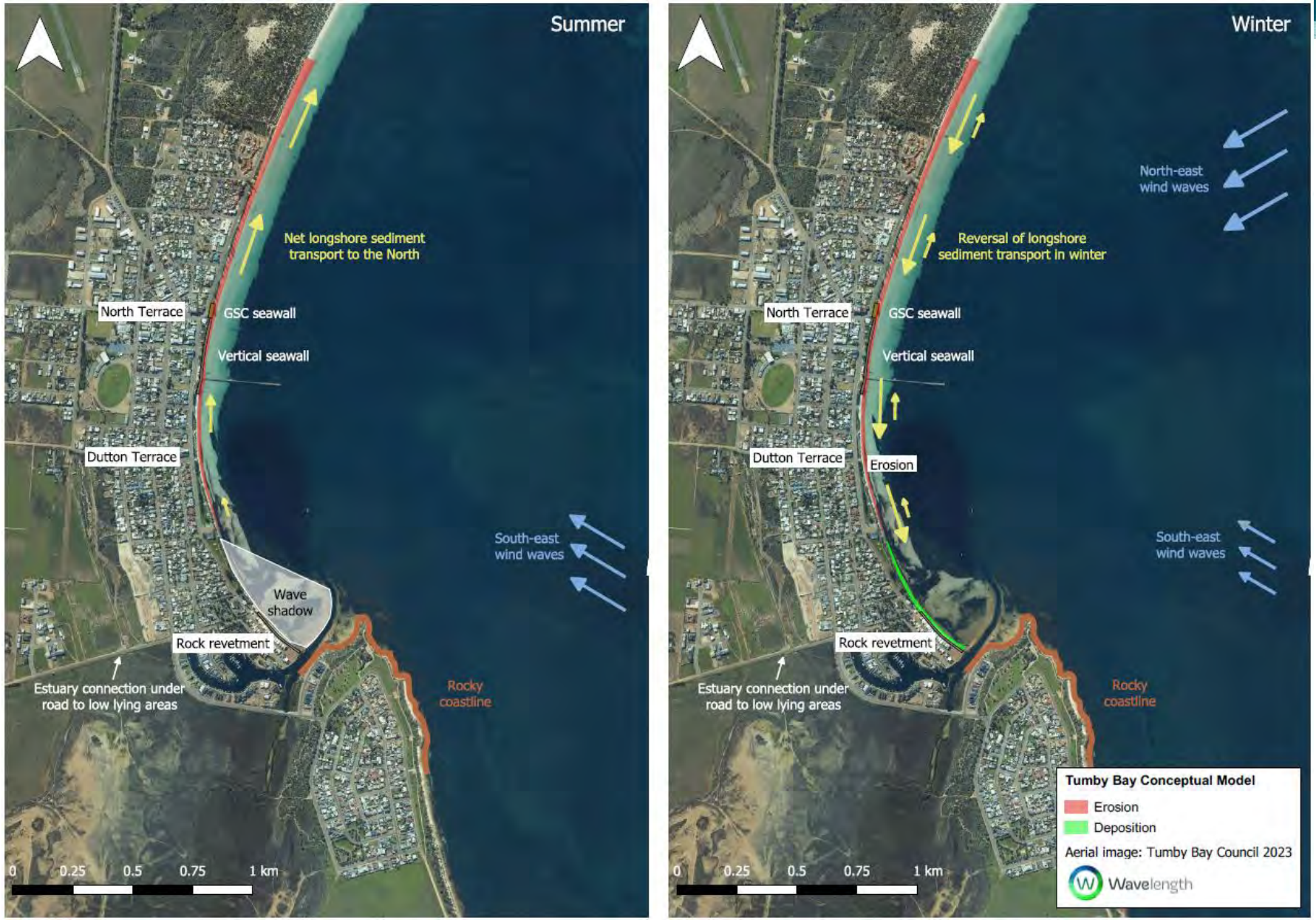
Figure 5: Overview of coastal processes and subsequent coastal management issues around the Tumby Bay township area
